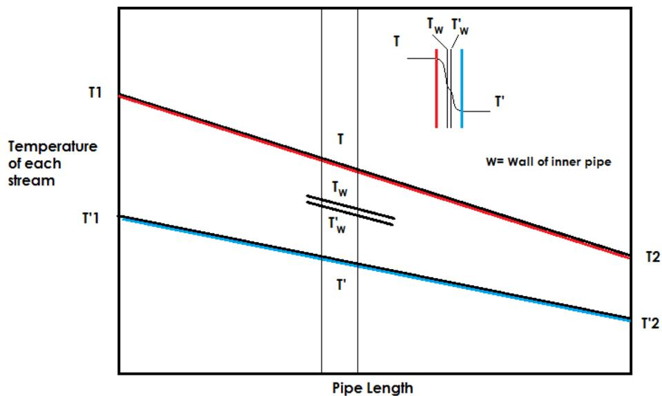
From repeated studies of simple heat exchanger systems (pure counter-current flow) it has been determined that there is a linear gradient between the two sets of end temperatures.
